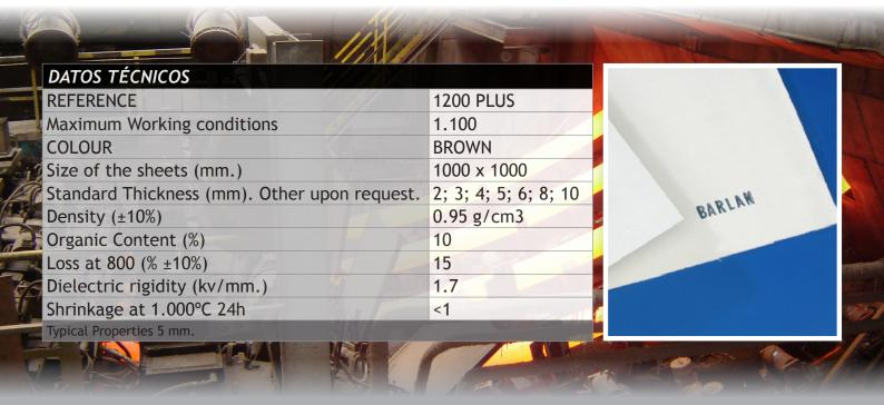
General insulation and heat protection. Also fire protection and electric insulation applications.
